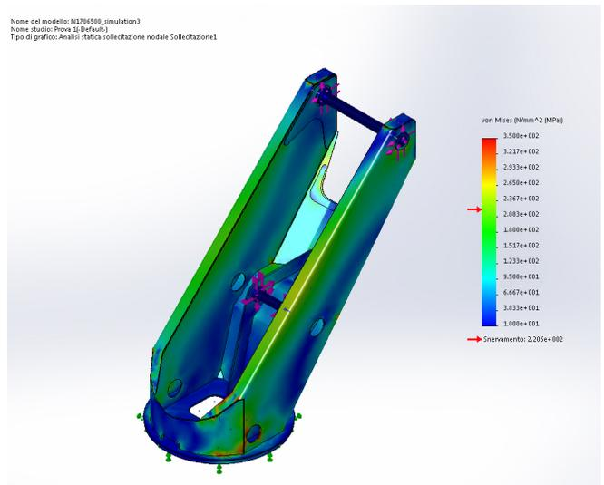
Using integrated SOLIDWORKS Simulation tools enables SOCAGE to achieve its overarching objectives of developing lighter, more compact aerial platforms while ensuring user safety.
